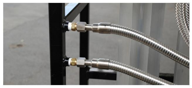
LEFT BLIND MANIFOLD IS FOR THE LIQUID OXYGEN HOSES. THESE HOSES HAVE THE SPIRAL WRAPPED STAINLESS STEEL HOSE GUARD. WHEN ONLY ONE LIQUID DEWAR IS USED LEAVE THE OTHER HOSE SEALED TO THE BLIND PLUG
